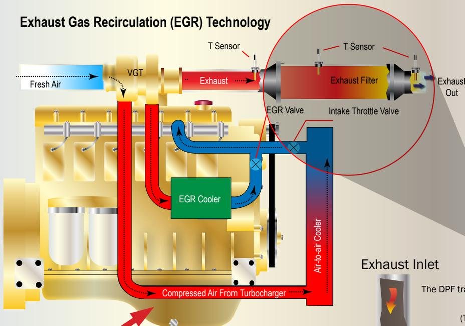
The diagram to the left demonstrates a diesel engine utilizing exhaust gas recirculation (EGR) and variable geometry turbocharger (VGT) technologies in off-highway applications such as diesel generator set systems. Interim Tier 4 solutions also add a catalyzed exhaust filter to meet emissions regulations.
